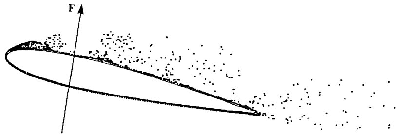
FIGURE 14.38 Simulation of the separated flow by the vortex tracing method. (Courtesy of P. R. Sparlat, 14.26 NASA Ames Research Center.) Reprinted with permission. Copyright AIAA.
